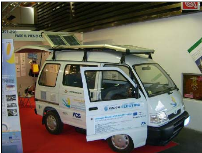
Fig. 3. A prototype of Hybrid Solar Vehicle with series structure developed at the University of Salerno.
